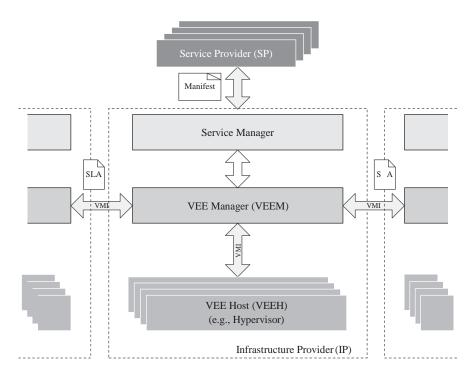
FIGURE 4.1.4. The RESERVOIR architecture: major components and interfaces.
