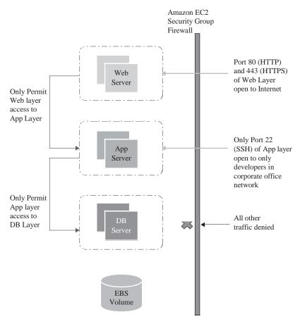
FIGURE 4.4.4. Securing your Web application using Amazon EC2 security groups.
