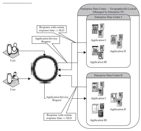
FIGURE 4.2.1. Hosting of applications on servers within enterprise's data centers.
