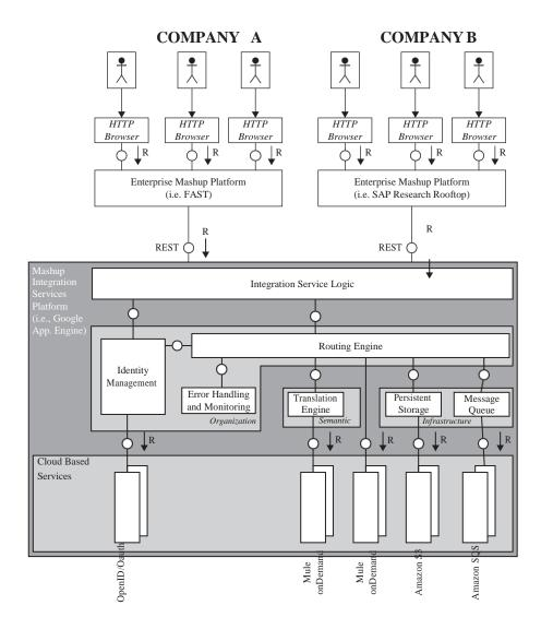
FIGURE 3.9. Cloudbased Enterprise Mashup Integration Platform Architecture.
