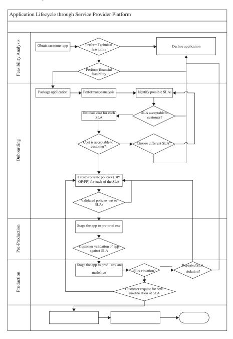
FIGURE 4.2.7. Flowchart of the SLA management in cloud.
