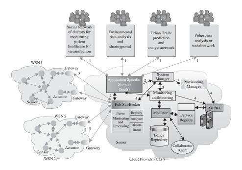
FIGURE 3.10. The Framework Architecture of Sensor—Cloud Integration.
