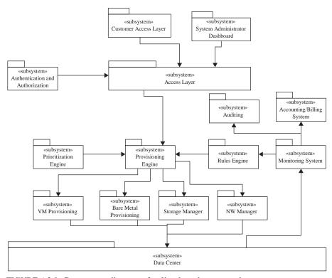
FIGURE 4.2.9. Component diagram of policy-based automated management system.
