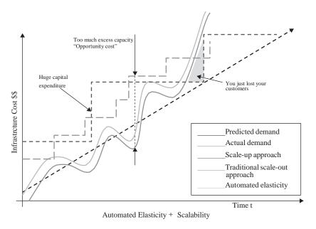
FIGURE 4.4.2. Automated elasticity.
