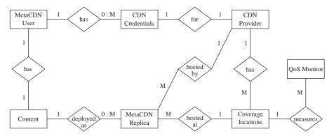
FIGURE 4.5.5. Entity relationship diagram for the MetaCDN database.
