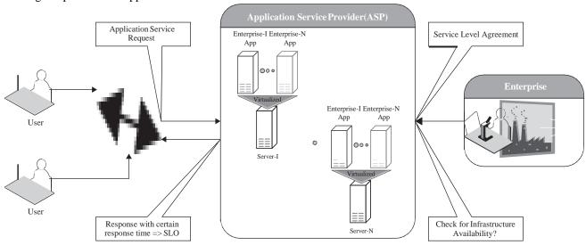
FIGURE 4.2.4. Shared hosting of applications on virtualized servers within ASP's data centers.
