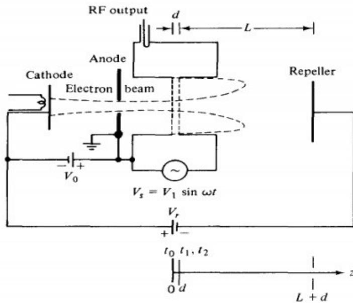
$t_0$  time for electron entering cavity gap at  $z = 0$
