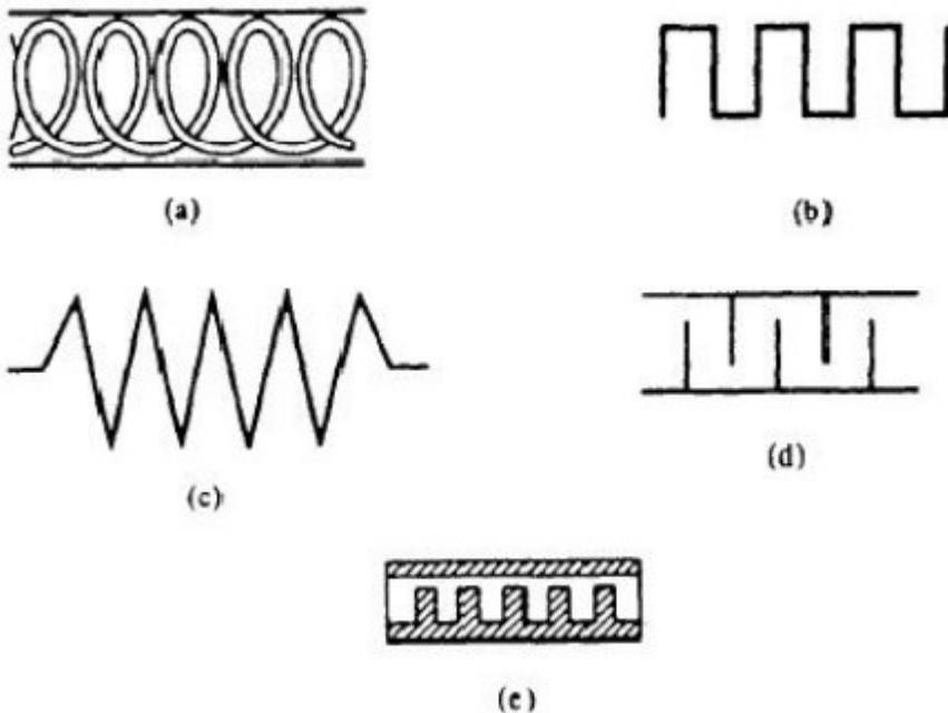
Slow-wave structures are special circuits that are used in microwave tubes to reduce the wave velocity in a certain direction so that the electron beam and the signal wave can interact. The phase velocity of a wave in ordinary waveguides is greater than the velocity of light in a vacuum.
