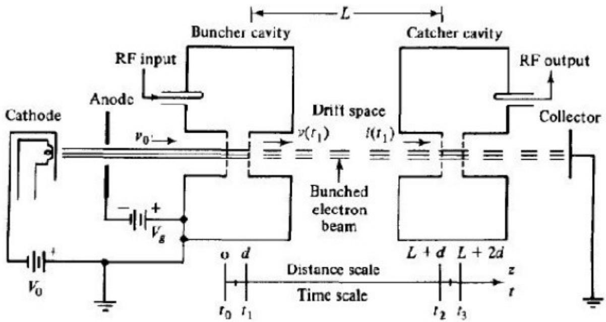
Figure 9-2-2 Two-cavity klystron amplifier.
