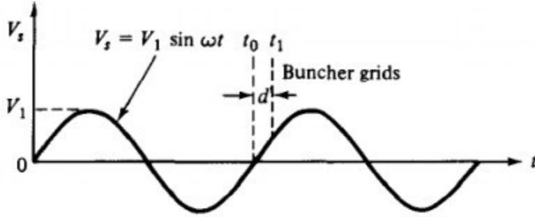
**Figure 9-2-6** Signal voltage in the buncher gap.
