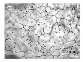
Optical Microstructure of a 99.5% pure aluminium
