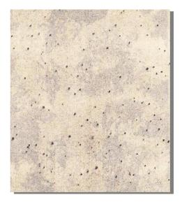
Scratch free surface after final polishing Magnification 50 X
