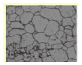
Optical Microstructure of a pure iron
