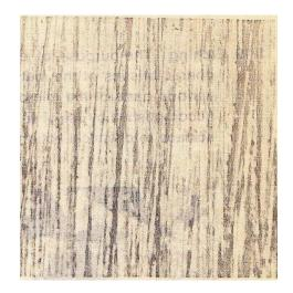
Surface after intermediate polishing on 4/0 Emery paper Magnification 100 X
