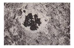
Microstructure of Malleable Cast Iron Temper Carbon is in the form of irregular aggregates.
