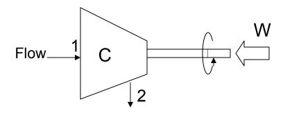
Applying First Law (steady-state, neglect heat transfer and  $\Delta PE$ )
