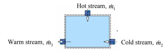
This type of heat exchanger consists of a vessel where a hot stream and cold stream of the same fluid are mixed and exit at an intermediate temperature through a single outlet.
