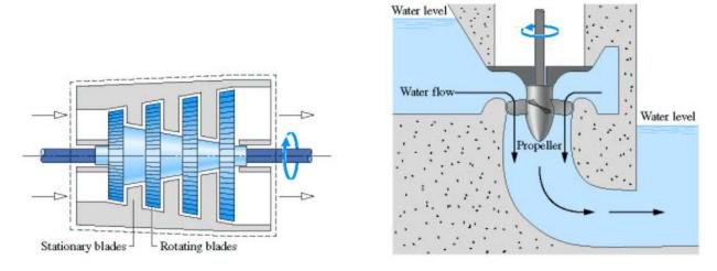
The rotating blades redirect the flow off axis, so you need a set of fixed blades that straighten out the flow before the next set of rotating blades
