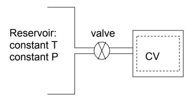
Considering the filling of a rigid tank of volume  $V_{cv}$  with a gas supplied at a constant pressure and temperature
