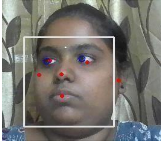
Fig 12.2.3 If the user wants to move the cursor towards left direction then the user should move the Anchor point to left
