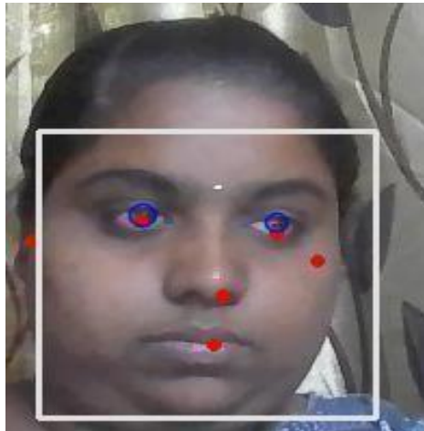
Fig 12.2.4 If the user wants to move the cursor towards right direction then the user should move the anchor point to right
