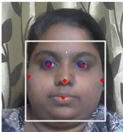
Fig 12.2.2 If the user wants to move the cursor towards downward direction then the user should move the Anchor point to down
