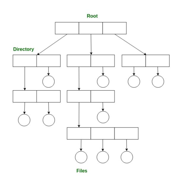
A tree structure is the most common directory structure. The tree has a root directory, and every file in the system has a unique path.
