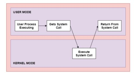
As can be seen from this diagram, the processes execute normally in the user mode until a system call interrupts this. Then the system call is executed on a priority basis in the kernel mode. After the execution of the system call, the control returns to the user mode and execution of user processes can be resumed.
