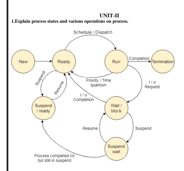
The process, from its creation to completion, passes through various states. The minimum number of states is five.
