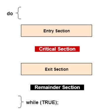
In the above diagram, the entry section handles the entry into the critical section. It acquires the resources needed for execution by the process. The exit section handles the exit from the critical section. It releases the resources and also informs the other processes that the critical section is free.
