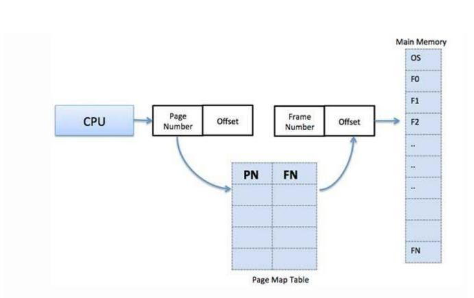
When the system allocates a frame to any page, it translates this logical address into a physical address and create entry into the page table to be used throughout execution of the program.
