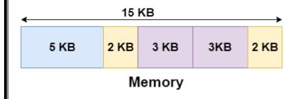
It is important to note that these partitions are allocated to the processes as they arrive and the partition that is allocated to the arrived process basically depends on the algorithm followed.
