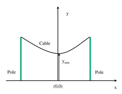
The cable has a uniform weight w (Newtons/meter or N/m or kg/sec<sup>2</sup>) per unit length. The differential equation, derived from force balance in the x and y directions, for the height y of the cable as a function of x is:
