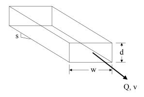
Figure 2: Flow in an open channel
