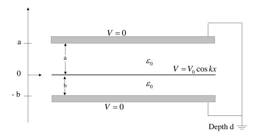
A sheet with electric potential distribution  $V(y=0) = V_0 \cos kx$  is placed at y=0, parallel and between two parallel grounded perfect conductors at zero potential at y = -b and y = a. The regions above and below the potential sheet have dielectric permittivity of free space  $\varepsilon_0$ . Neglect fringing field effects.
