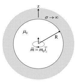
A point magnetic dipole  $\overline{m} = m_0 \overline{i_z}$  is placed at the center of a free space spherical cavity of radius R within a perfect conducter  $(\sigma \to \infty)$ .
