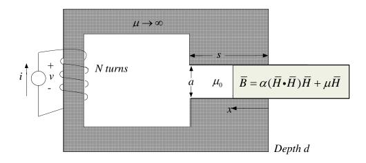
A slab of nonlinear magnetic material with  $\overline{B} - \overline{H}$  relationship
