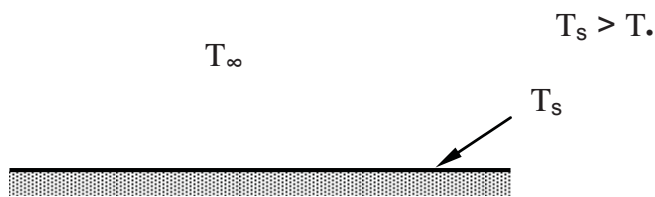
Figure 3-12 Natural convection over a horizontal flat plate
